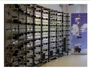
Groups of transmitters and receivers at a base station are coupled to a single antenna with a multicoupling network thus greatly improving station efficiency.
